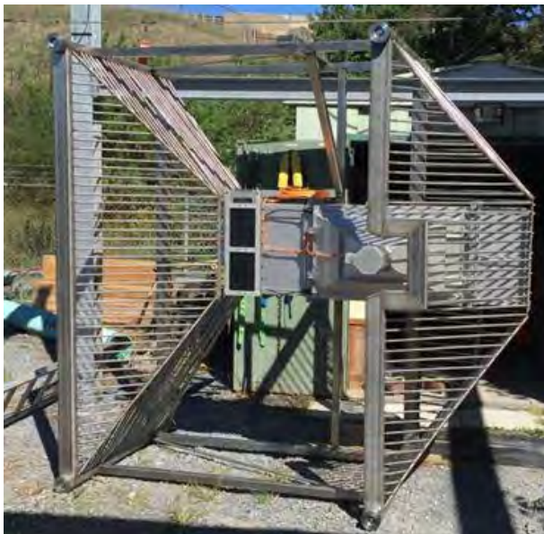
FIG. 9.7.3. VAKI Riverwatcher fish counter and frame designed for the Ganaraska Fishway.
