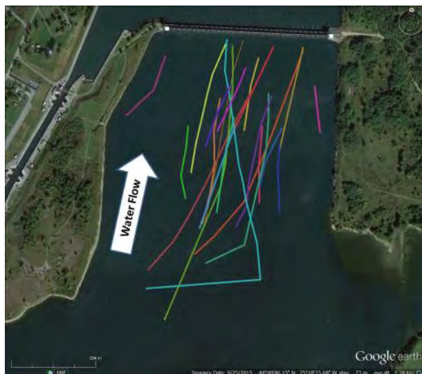
FIG. 8.3.7. Image of Iroquois Water Control Structure in the upper St. Lawrence River. Lines represent the track of tagged eels (as detected by acoustic receivers) during September to December 2016. Locations of the eels were calculated from receiver data by VPS ( https://vemco.com/products/vps/ ).
