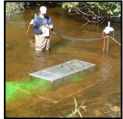
A student researcher uses dyes to identify stream flow regimes and pheromone concentrations during research trials to identify better sea lamprey management techniques.
