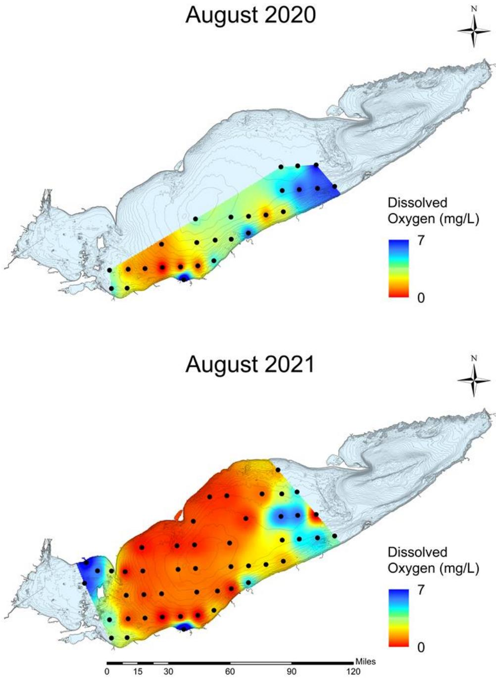
Figure 7: GLATOS stations equipped with data loggers during 2020 and 2021 (black dots). As an example, average dissolved oxygen distribution in the hypolimnion was interpolated (with IDW) and is plotted as a heat map.
