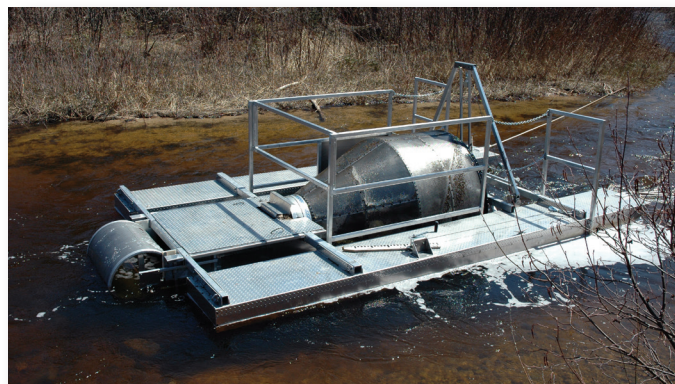
A new, experimental screw trap being tested on Carp Lake Outlet, Michigan.
