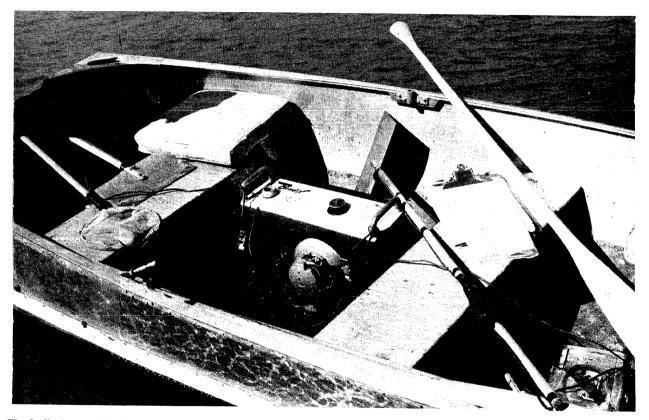
Fig. 8. Equipment developed in 1958 for collecting ammocetes from Canadian tributaries of the Great Lakes. Note the compact, gasoline-powered electric generator; two galvanized steel electrodes on wooden dowels (one with micro switch sealed in a rubber cover); and a dip net for collecting specimens.
