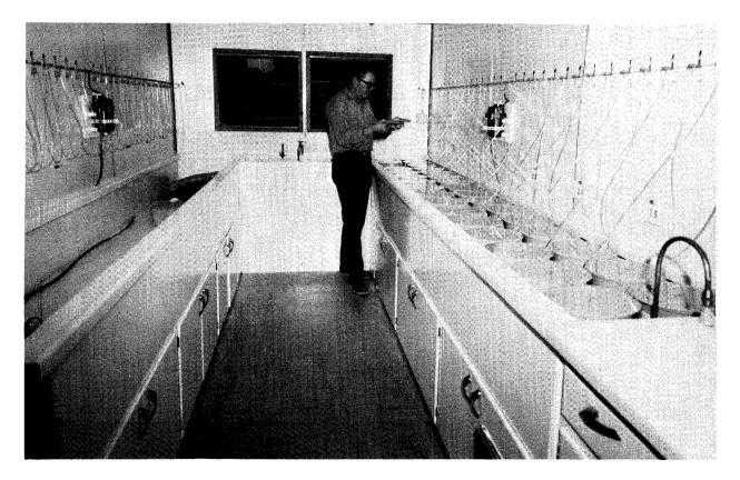
Fig. 11. Mobile bioassay laboratory. Lamprey ammocetes and fingerling rainbow trout are placed in the test containers and exposed to a range of lampricide concentrations. The time to death at each concentration is noted.
