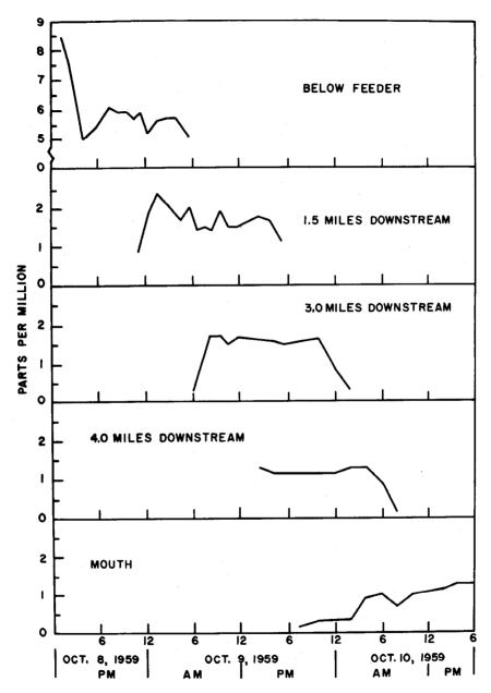
Fig. 15. TFM concentration at five locations in the Traverse River, Houghton County, Michigan, as the lampricide moved downstream during a treatment in October 1959. Minimum lethal concentration was 1.0 ppm and maximum allowable concentration, 4.0 ppm.
