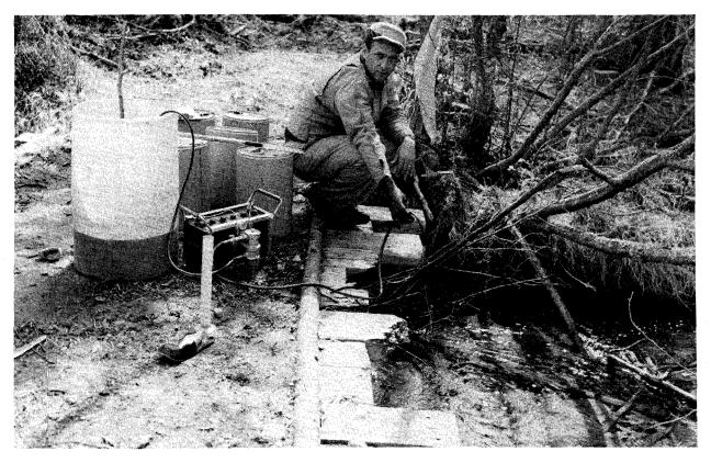
Fig. 14. Application of lampricide into a stream with a battery-operated fuel pump feeder equipped with calibrated orifice that controls rate of flow.
