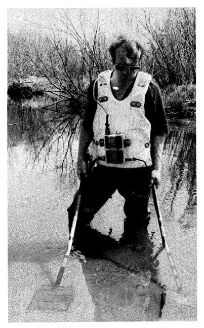
Fig. 9. Collecting ammocetes with a transistorized back-pack shocker.
