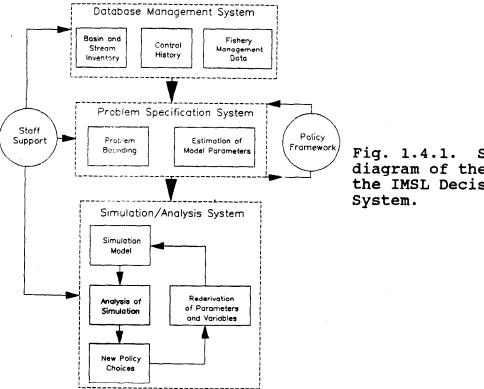
Schematic diagram of the structure of the IMSL Decision Support
