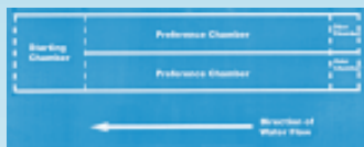
Dr. Li's two-choice maze used to examine the behavioral responses of adult sea lamprey to pheromones (top). The above figure illustrates the design of the device.
