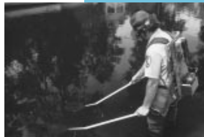
Biologists wear backpack electro-fishing gear to stimulate larval sea lampreys out of their burrows. The data are used to measure larval sea lamprey abundance in Great Lakes streams and tributaries.
