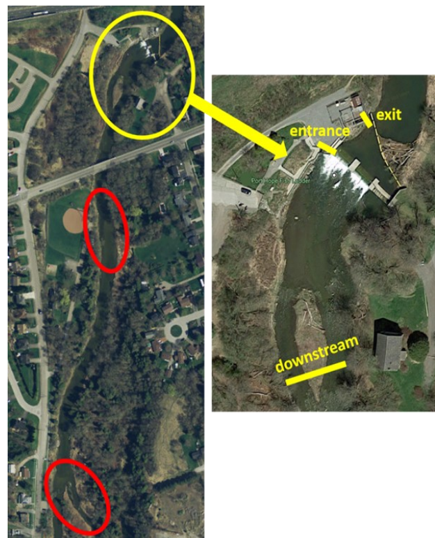
FIG. 9.9.1. Left: Ganaraska River tagging reach with red circles depicting where most fish tagging occurred. Right: Locations of antennas around and within the fishway.
