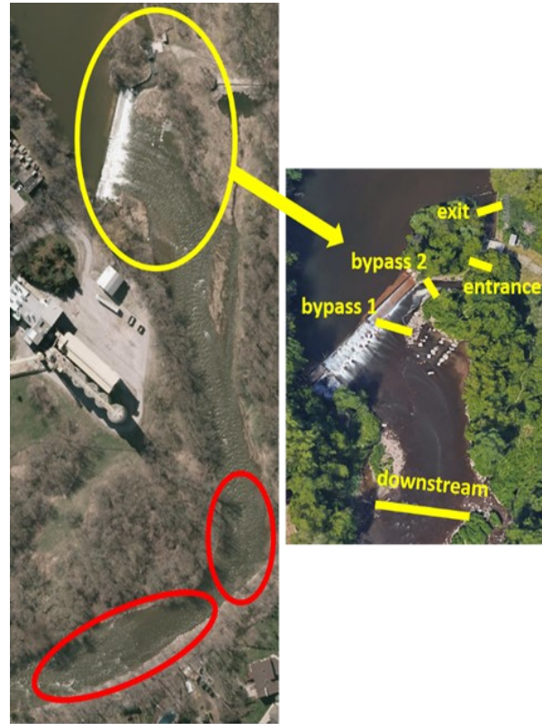
FIG. 9.9.2. Left: Credit river tagging reach with red circles depicting where most fish tagging occurred. Right: Locations of antennas around and within the fishway. Bypass antennae were decommissioned due to interference with the entrance and exit antennae.
