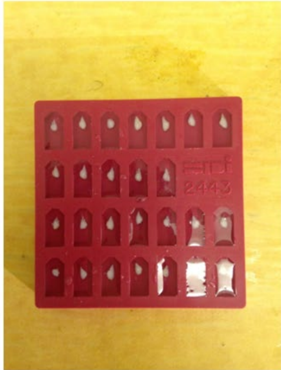
Filled embedding mold
