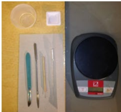
Materials for weighing/mixing/transferring epoxy
